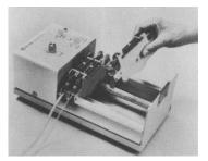
• Manostat's multichannel Cassette Pump can handle up to 20 channels with one basic drive unit. The unit has solid state control to provide constant flow and infinitely variable pumping rates with no variation from forward to reverse, the firm says. Information: Monostat Corp., 519 8th Ave., New York, NY 10018.
