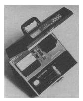
• Hach Chemical Company says its new self-contained nephelometer, the PortaLab Turbidimeter, can be operated on rechargeable nickel cadmium batteries or standard 110 AC power. Readings are available within five seconds from the 10-pound instrument. Information: Hach Chemical Co., PO Box 389, Loveland, CO 80537.
