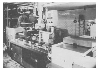
• Len E. Ivarson is offering the Benhil 8346 fully automatic, high-speed filling and wrapping machine to handle margarine, butter, lard, shortening and other edible fats in package sizes from one to five pounds. The wrapper is formed with a plunger before product filling. Up to 30 five-pound packages or 50 one- or two-pound packages can be filled per minute. Information: Len E. Ivarson, Inc., 3100 W. Green Tree Road, Milwaukee, WI 53223.
